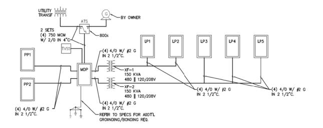
Figure 3. One-Line Diagram
