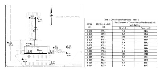
Figure 4. Boring Test Locations
